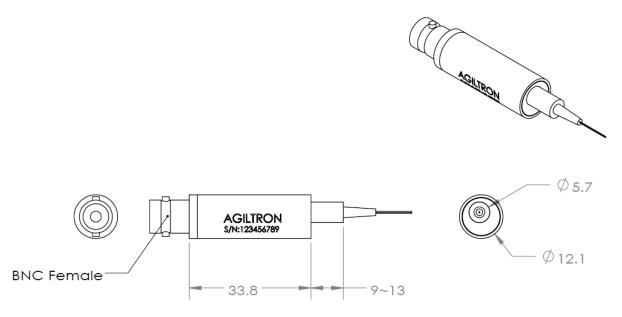
dimensions tolerance to be +/-0.2mm
